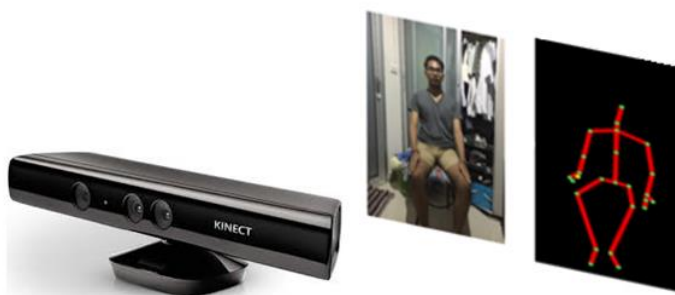
Figure 1 Kinect camera and human joints extracted from Kinect
