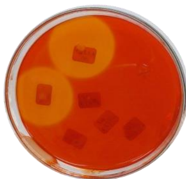
Figure 1 Clear zone formation by bacterial isolate A023 on an MSM agar plate using a spot diffusion assay. The plate was incubated at 37°C for 2 days and stained with Congo red.
