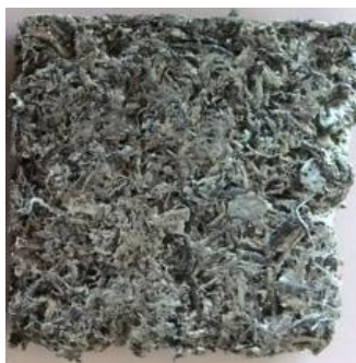
Figure 2 a) WHF after mixing with NRL b) Mixed WHF after oven-drying
