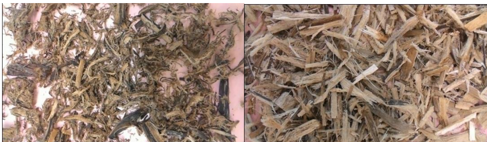
Figure 1 a) WHF after ground into crusher b) WHF after boiled in 10wt% sodium hydroxide and dried.
