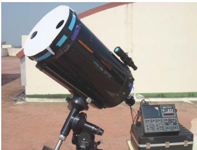
Figure 1 The equipments of the DIMM method for seeing test at Samorkraeng Mountain
