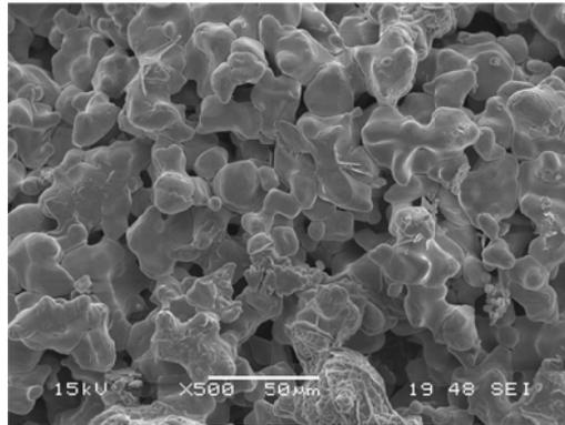
**Figure 2** The microstructure of Ba(Ti<sub>0.95</sub>Zr<sub>0.05</sub>)O<sub>3</sub> taped products at 500 x.
