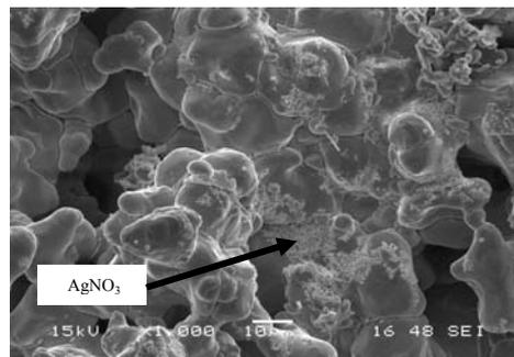
**Figure 4** The microstructure of  $\text{Ba}(\text{Ti}_{0.95}\text{Zr}_{0.05})\text{O}_3$  taped products with  $\text{AgNO}_3$  adsorption at 1000 x.
