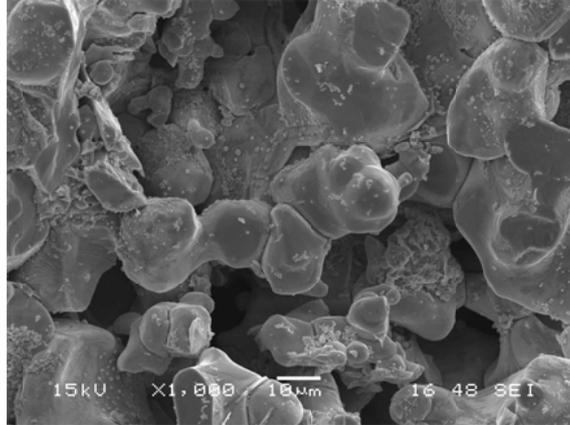
**Figure 5** The microstructure of Ba(Ti<sub>0.95</sub>Zr<sub>0.05</sub>)O<sub>3</sub> pellet ceramics with AgNO<sub>3</sub> adsorption at 1000 x .
