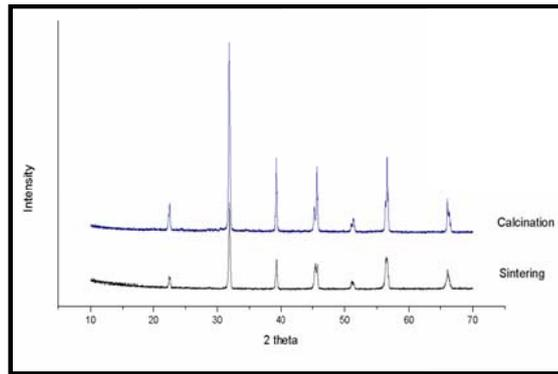
**Figure 1** X-ray diffraction patterns of  $\text{Ba}(\text{Ti}_{0.95}\text{Zr}_{0.05})\text{O}_3$  calcined powder and sintered ceramics.
