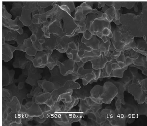
**Figure 3** The microstructure of Ba(Ti<sub>0.95</sub>Zr<sub>0.05</sub>)O<sub>3</sub> pellet ceramics at 500 x.
